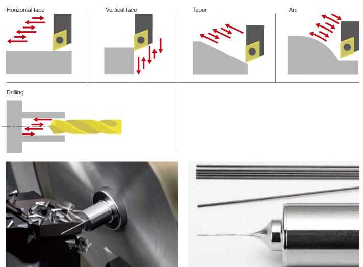
Micromachining leaving 0.2 mm dia. pin
