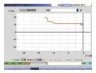
Vibration cutting path display "x" indicates the cutting position, which can be changed either with the tab key or with the manual pulse handle.
