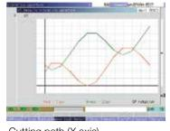
Cutting path (X axis) This displays the cutting paths for the first and second rotations. The sections where the lines intertwine are where the chips are broken up.
