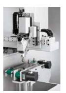
Pallet Conveyor This is a conveyor suited to the feed/conveyance of irregularly shaped products, and precision parts that must not be scratched.
