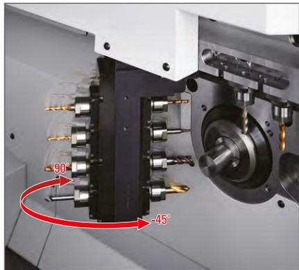
**U32B (B axis: rotary tools on the gang tool post)**
