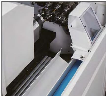
**Workpiece conveyor equipped as standard**
