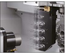
Features a B axis for rotary tools on the gang tool posts of Type XII machines as standard; capable of working on both spindles it can be programmed over a  $135^{\circ}$  range from 90° to -45°.
