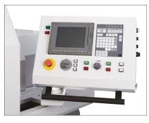
Adjustable operation panel By swiveling the adjustable operation panel, you can perform operations while watching the machining area.
