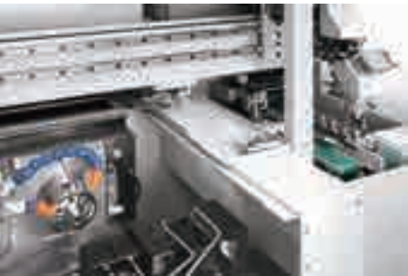
Gantry loader with high-speed travel of 154 m/min. on the X axis.
